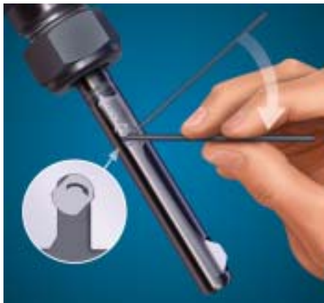
Lock the flex arm back into place with a simple 1/8 clockwise turn of the locking screw.
