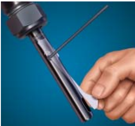
Insert the tab at the end of the blade into the groove of the adjusting screw. Lower the slot of the blade over the lock screw.
