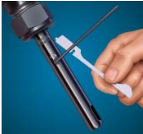
Once in the unlocked position the blade can be pulled up and out of the holder.
