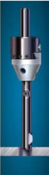
The tool is lowered into the hole with the head adjusted so that the arbor has approximately .004" clearance.
