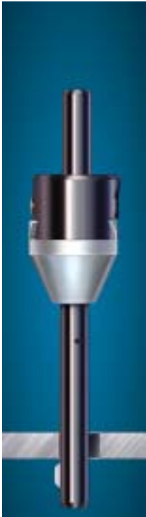
The tool is rapid fed through the part so the blade is beyond the burr by approximately .040". The feed direction is then reversed and fine fed back into the part until the blade is collapsed into the holder.
