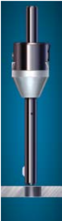
The tool is rapid fed out of the part and is ready to proceed to the next hole.
